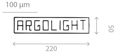
Fig. 13: Schematics of the Argolight logo. All dimensions are in \mu\text{m} .
