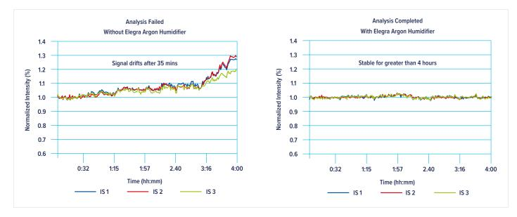
The graphs above demonstrate the benefit of using the Elegra with the real-world application of analyzing fusion samples with 0.5% lithium metaborate by ICP-OES. All three internal standard lines monitored began to drift quickly when no Elegra was used, while their responses were very stable with the Elegra installed.
