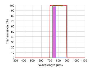
Fig 5: A tunable bandpass filter created with VersaChrome TLP and TSP filters, matched with the appropriate full spectrum blocking filter. The effective composite bandpass filter created is shown in solid purple.
