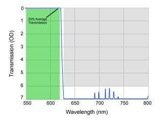
Figure 4: VersaChrome short-wave pass tunable edge filters maintain high transmission and deep blocking, even at AOI = 60°.
