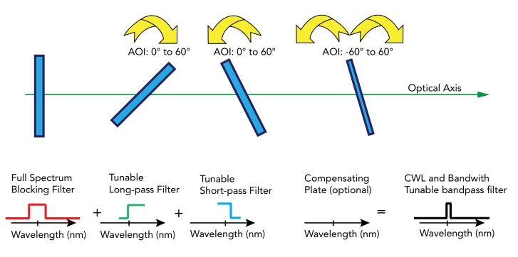
Figure 2: Combining VersaChrome Edge Tunable Filters will allow any single-band filter in the visible or near infrared to be created.
