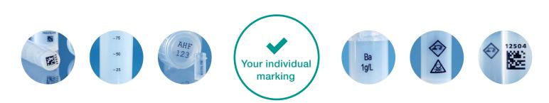
The marking options are manifold and can be choosen individually: Lettering, numbers, barcodes, 2D codes (DataMatrix, QR-Code), volume marks, single-color pictograms, warning and hazard symbols and logos. This allows you to realize labels that are machine-readable and support the automation process in your laboratory. The individual motifs can have a size of up to 70 x 70 mm.
