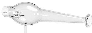
The Lotis™ HE spray chamber directly couples to the ICP-MS torch, providing the highest transport efficiency and excellent washout between samples.
