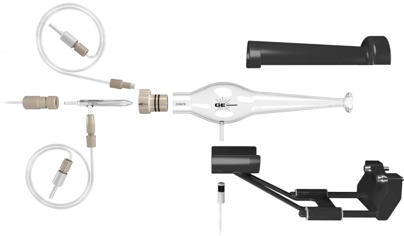
Originally designed as a highly efficient single-cell sample introduction system, Glass Expansion's HE-SIS has been redesigned to provide superior performance across a wide variety of applications, including single-cell, single particle, nanoparticle, and low-volume sample studies, with up to 95% transport efficiency.
